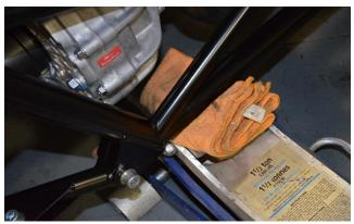
Be sure to position the jack on the left hand side of the car near the transmission on the rear most tube on the chassis. We place a thick cloth or towel folded over on the chassis to prevent scuffing the finish. (Cont.)
